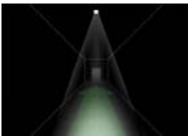
Escape route illumination with asymmetric optics
