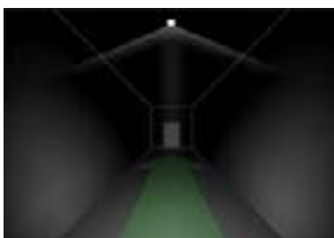
Escape route illumination with symmetric optics
